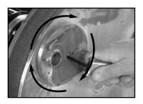
Must rotate clockwise towards the spring leg. If it rotated in reverse, damage could be caused to spring. Running a short distance on a smooth floor to remove glaze from spring should be ok but not to be consistently run that way.
